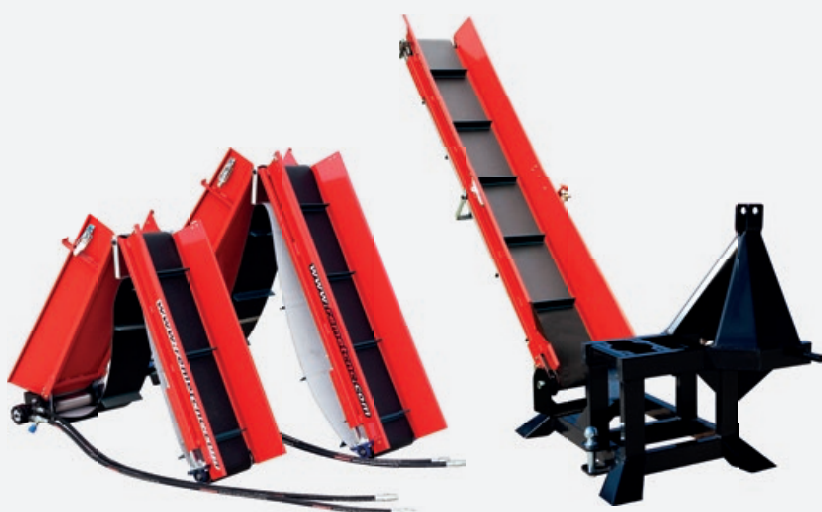
BELT CONVEYORS FOR WOOD CHIPPERS WITH HYDRAULIC DRIVE: Length 160 cm, width 25 cm for R/RP-100 Length 230 cm, width 25 cm for R/RP-120 Length 300 cm, width 30 cm for R/RP-150 Length 400 cm, width 40 cm for RP-200 Length 160 cm, width 25 cm, with frame RP-100 Length 230 cm, width 25 cm, with frame RP-120 Length 300 cm, width 30 cm, with frame RP-150 Length 400 cm, width 40 cm, with frame RP-200
