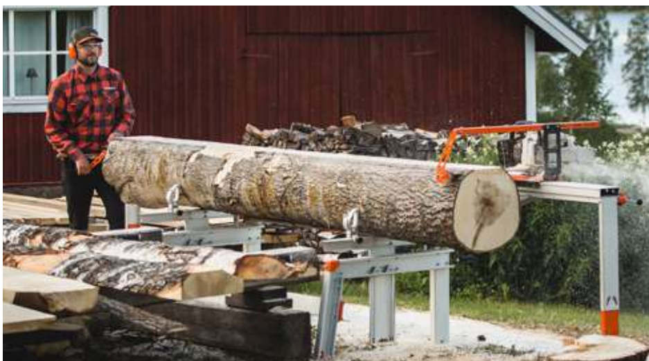
• The remote feeding is easy to mount on your chainsaw and makes sawing easier.
