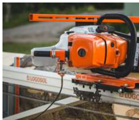
• The remote feeding is easy to mount on your chainsaw and makes sawing easier.
